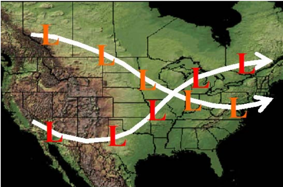
Figure 18: Typical "storm tracks" that influence the wind resource of the Upper Midwest. The bold Ls represent surface cyclone positions as they move along the track.
