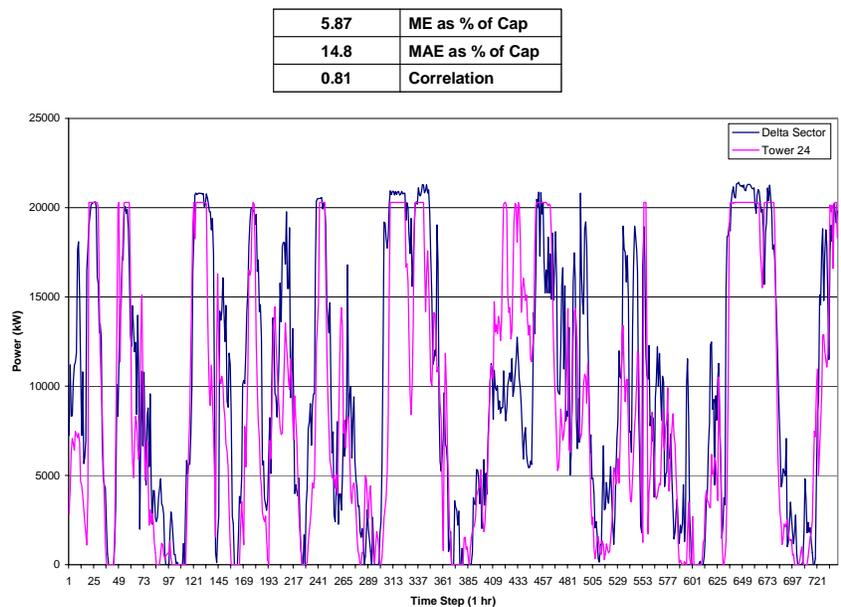
Figure 3: Comparison of simulated wind generation data to actual measurements for a group of wind turbines at Lake Benton, MN on the Buffalo Ridge
