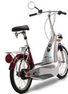
**Electric-assisted bicycles** have a saddle and operable pedals, no more than three wheels, and an electric motor of up to 1,000 watts. The motor must disengage during braking and have a maximum speed of 20 miles per hour (whether assisted by human power or not). Electric-assisted bicycles are a subgroup of motorized bicycles.
