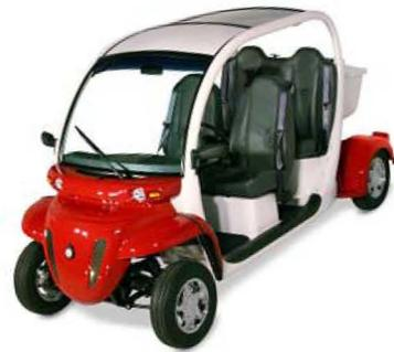
NEVs have primarily been produced for niche uses such as military bases and retirement communities, but their use is widening. The largest U.S. market is in California. The vehicles are rechargeable through the electrical grid and have a range of between 30 to 75 miles before needing to recharge. Models come in styles ranging from two-seaters to small-scale trucks, weighing 1,000 to around 1,500 pounds. Prices start at about \$8,000.
