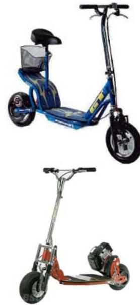
Types include both gas and electric motors. Electric models generally have a top speed below 15 miles per hour and a range of up to 20 miles. Models with gas engines commonly range from 25 to 50 cc (1.5 to 2.5 horsepower), and can have a top speed of over 30 miles per hour.
