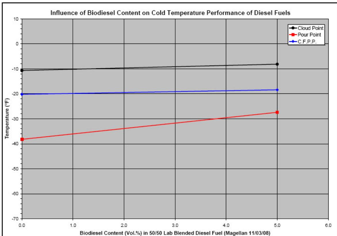
**Table 1. Cold Temperature Test Performance of Biodiesel Blends (in Study to Date)**
