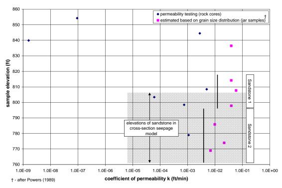
Figure 5.2 Permeability data for the Jordan Sandstone at Rapidan Dam.
