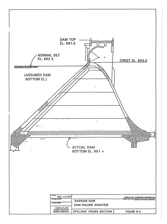
**Figure 1 Dam Cross Section**
