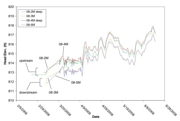
Figure 3.3 Detail of readings from piezometers installed at "deep" locations.
