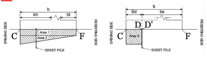
Assume axes runs along the heel at point c "into the board". The moment at the heel is positive using the right hand rule, therefore, how the picture is drawn, the moment is positive clockwise.
