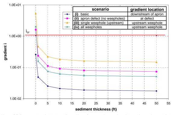
Figure 5.5 Computed vertical hydraulic gradients for several scenarios with varying sediment thickness.
