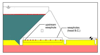
Figure 5.4 Weepholes were modeled by applying a head boundary condition (tailwater) at the weephole location.
