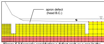
Figure 5.3 Scenario considering a defect such as a gap in the downstream apron.
