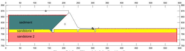
Figure 5.1 Seep/W model of the Rapidan Dam.
