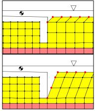
Figure 5.2 Scenarios considering a gap due to erosion downstream of the apron sill.
