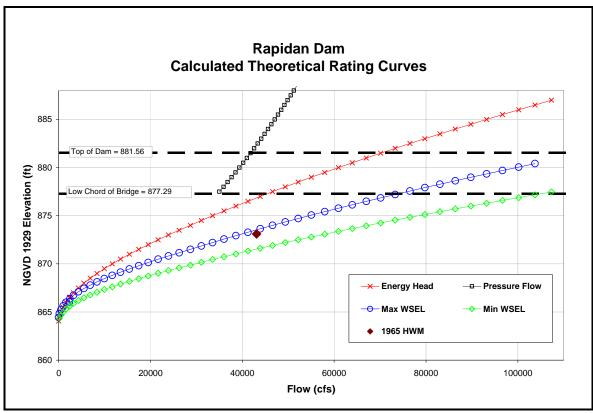
Figure 4: Theoretical rating curves for Rapidan Dam spillway.
