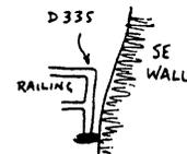
D728 1208.97 + on wall Chiseled + on northwest wall of passage to Formation Room, 3 ft above floor, in bed DL1, at northeast end of grate over fissure in floor.
