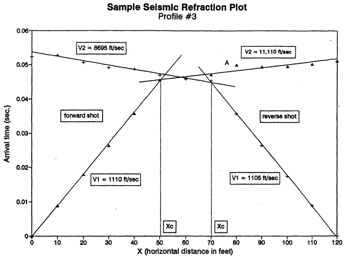
Figure 3: Example of travel-time graph for seismic refraction profiles.
