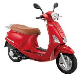
Motor scooters differ from motorcycles in a couple of ways. The standard design is step-through with a low platform for the operator’s feet, and the engine is most often located underneath
