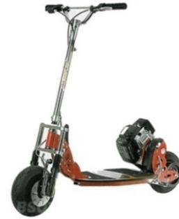
The devices are usually lightweight platforms with two small wheels, having a design similar to a skateboard but with a motor as well as steering and acceleration control via handlebars. Braking is from a hand brake on the handlebar or by using a foot-operated rear-wheel brake. Some models have a seat or saddle that sometimes is removable, which is found on more powerful and expensive offerings. Many motorized foot scooters weigh around 20 to 65 pounds, although heavier designs are available.
