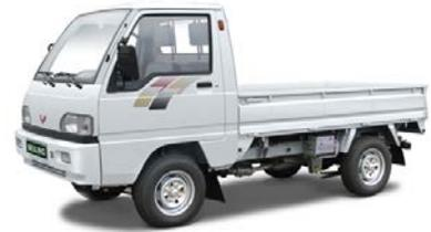
Although they come in different forms, the typical mini-truck design is an open flat bed behind a small enclosed cab for the driver and one passenger. Features can include air conditioning and all-wheel drive. They have traditionally been imported for off-road uses like recreational off-road activity, agricultural work on farms and ranches, at construction sites, in industrial parks, and grounds maintenance.
