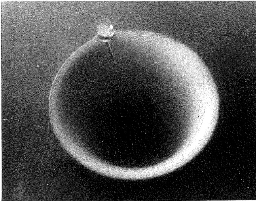
Photo 11. Viscous dimple which occurred in place of a bubble entraining vortex, or an air entraining vortex, at  $Fr \leq 0.85$ .
