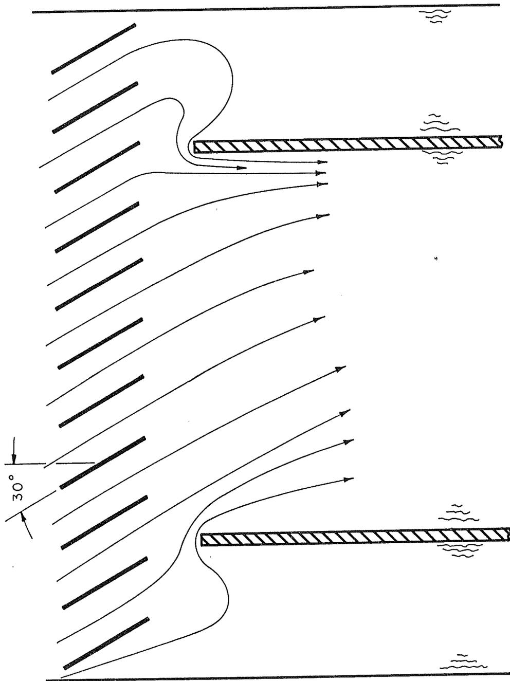
Fig. 24. Dye streaklines for  $S/D = 4.39$ ,  $F = 3.59$ ;
