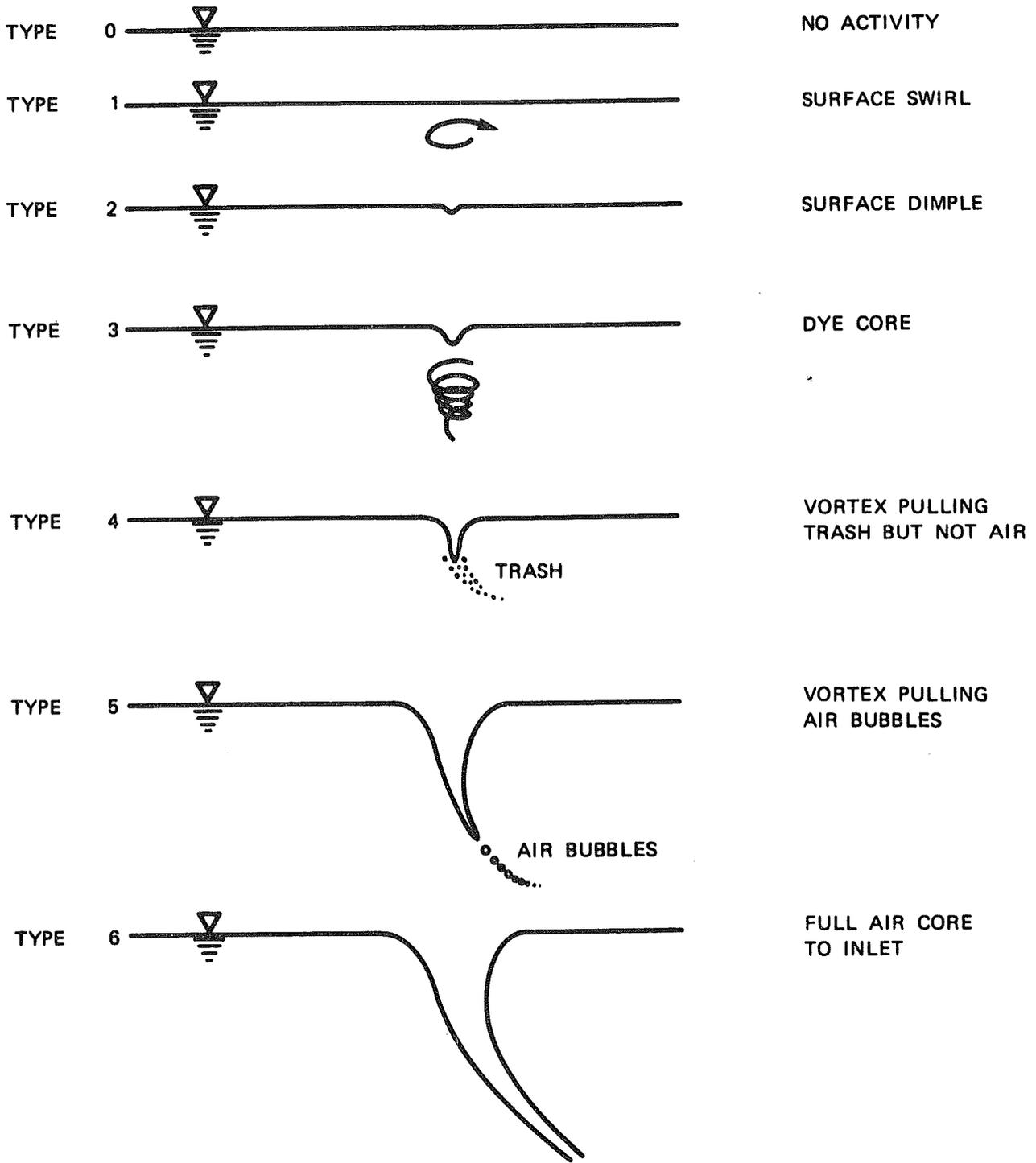
Fig. 25. Vortex strength scale used by Durgin and Anderson [25] for classification of free surface vortices at intakes.
