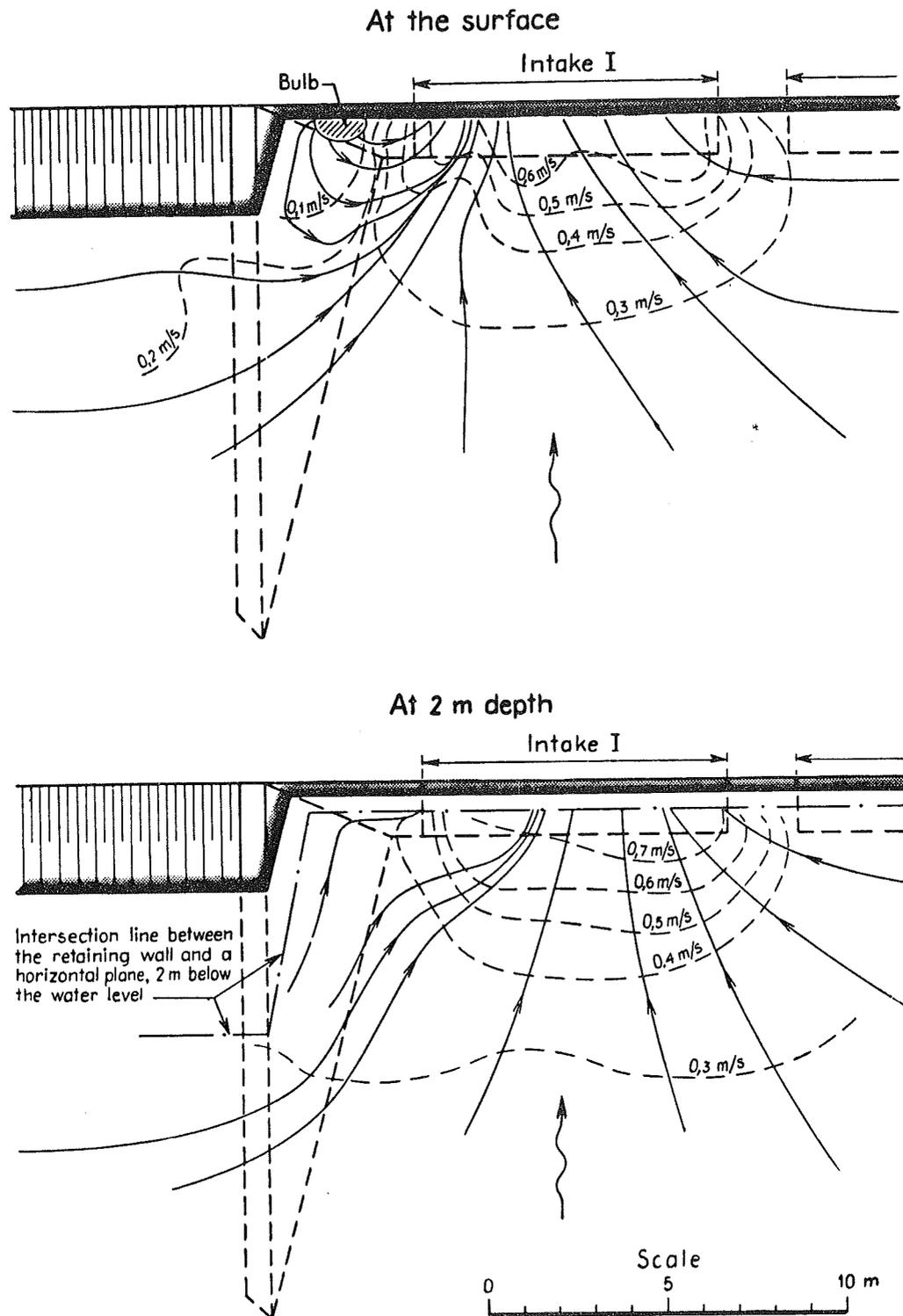
Fig. 16. Åtorp Power Plant streamlines and velocities in front of intake I with a discharge of  $37 \text{ m}^3/\text{s}$ , unit II being closed, taken from Rahm [3].
