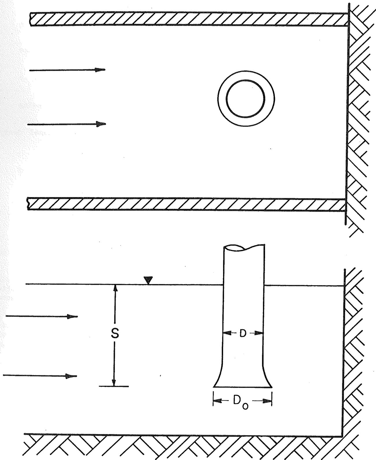
Fig. 2. Vertically inverted intake configuration.
