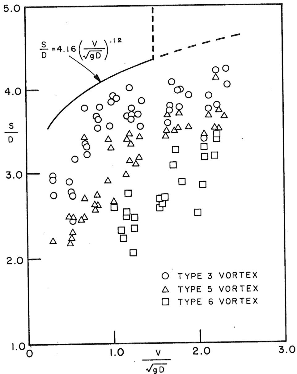
Fig. 28. Dimensionless submergence versus intake Froude number for  $15^\circ$  vane angle and  $L/W = 1.13$ .
