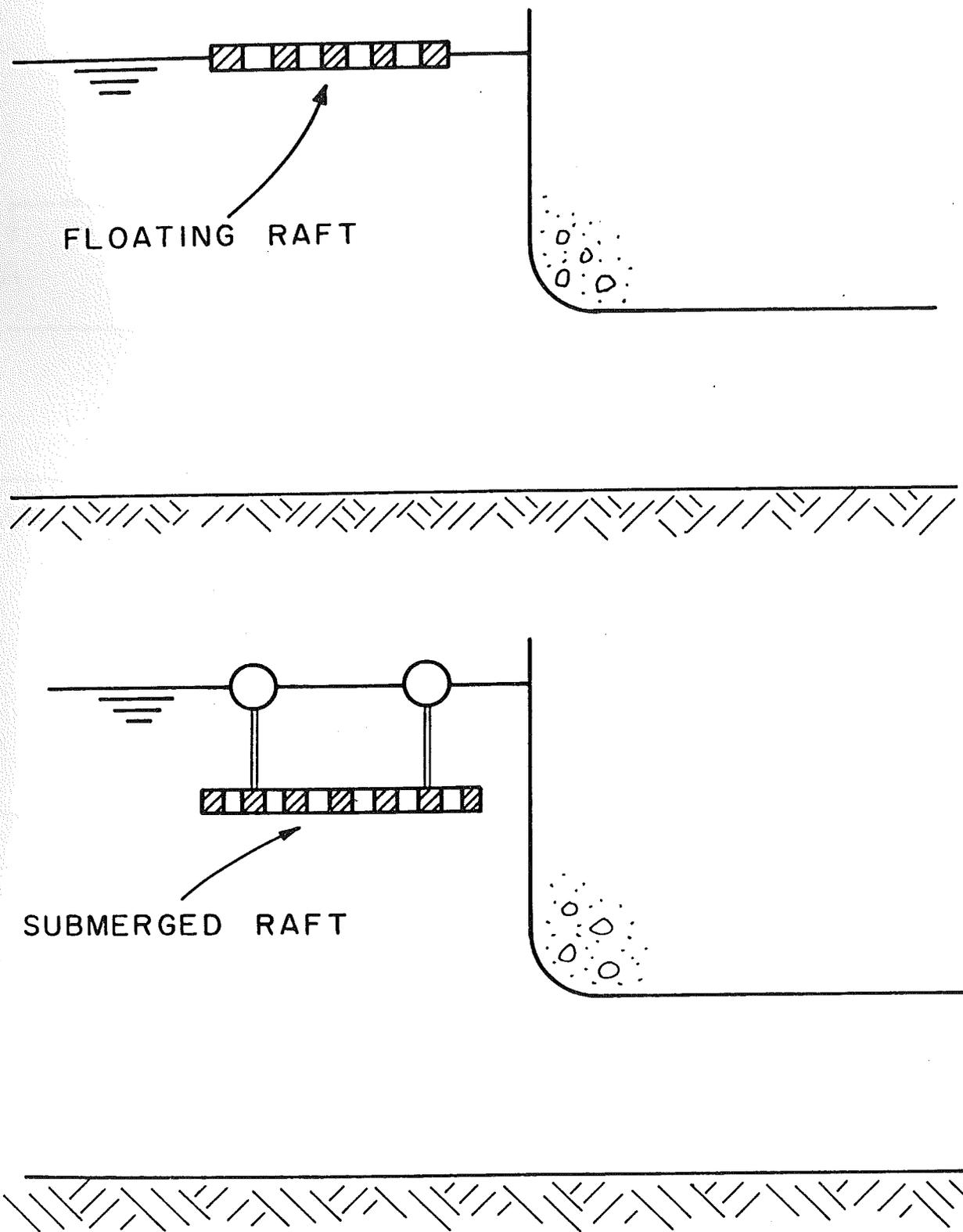
Fig. 5. Floating and submerged raft vortex suppressors.
