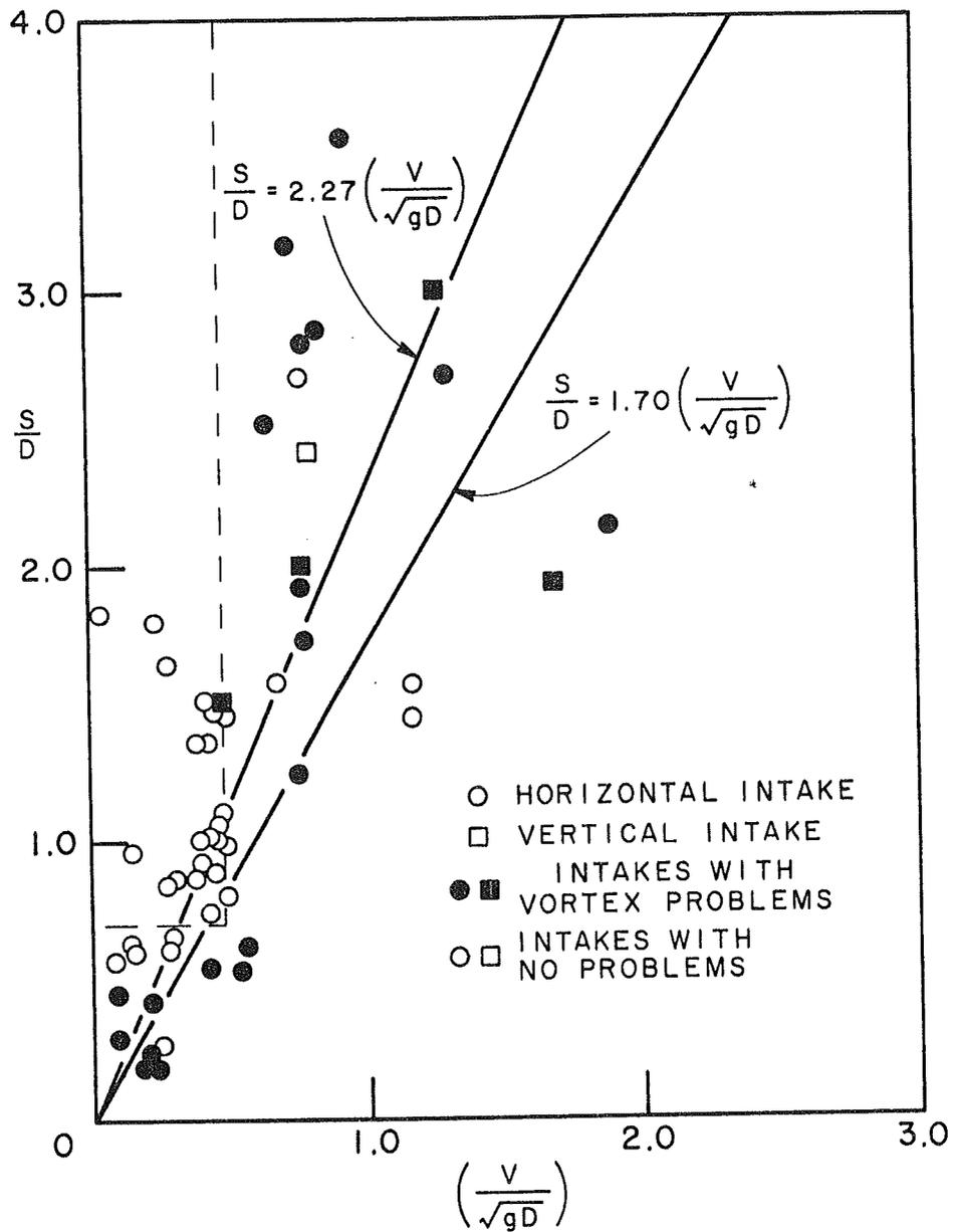
Fig. 19. Dimensionless plot of data obtained from existing intakes, field installations and model studies.
