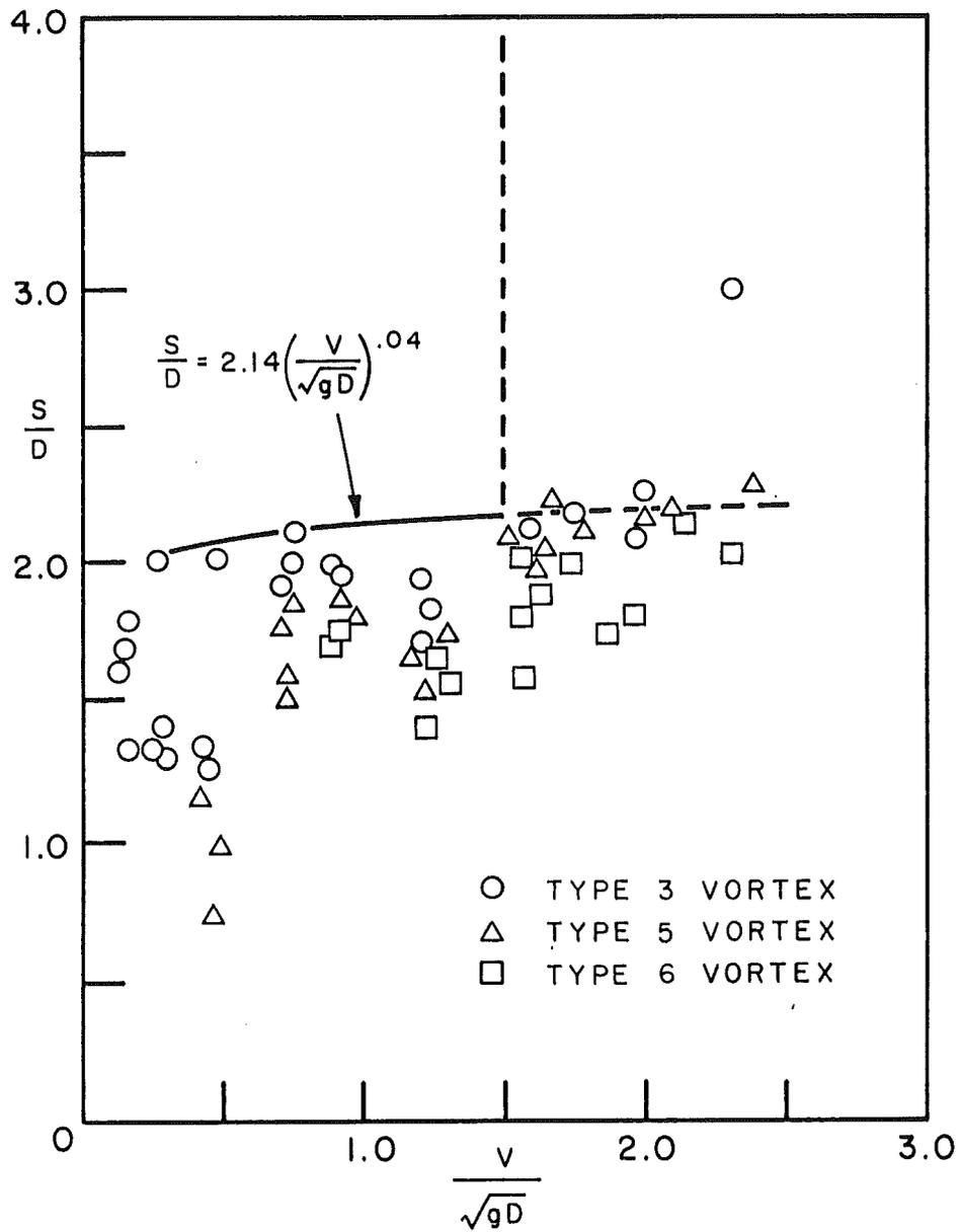
Fig. 34. Dimensionless submergence versus intake Froude number for  $0^\circ$  vane angle and  $L/W = 3.56$ .
