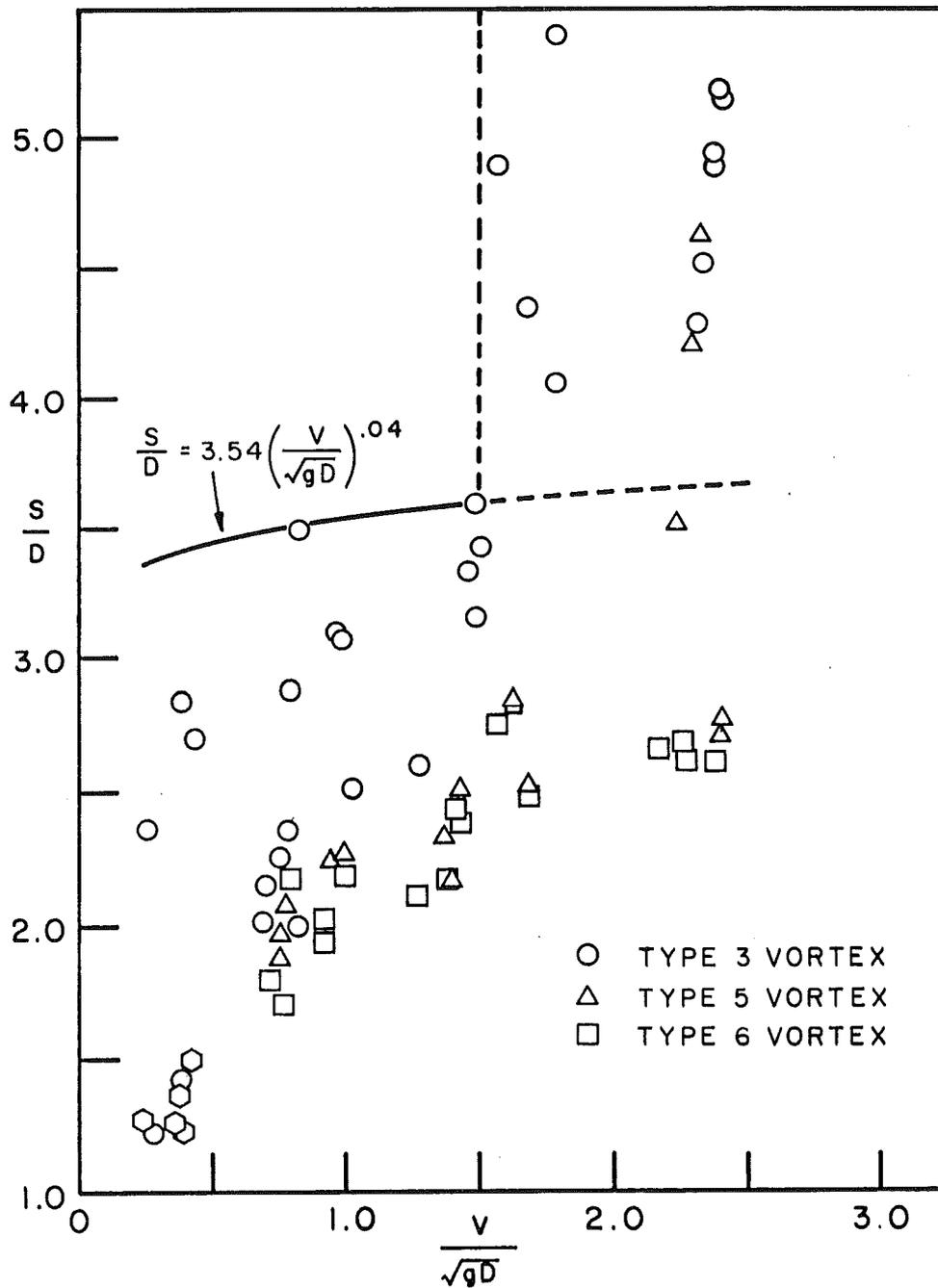
Fig. 36. Dimensionless submergence versus intake Froude number for  $15^\circ$  vane angle and  $L/W = 3.56$ . Hexagon symbol indicates viscous dimple.
