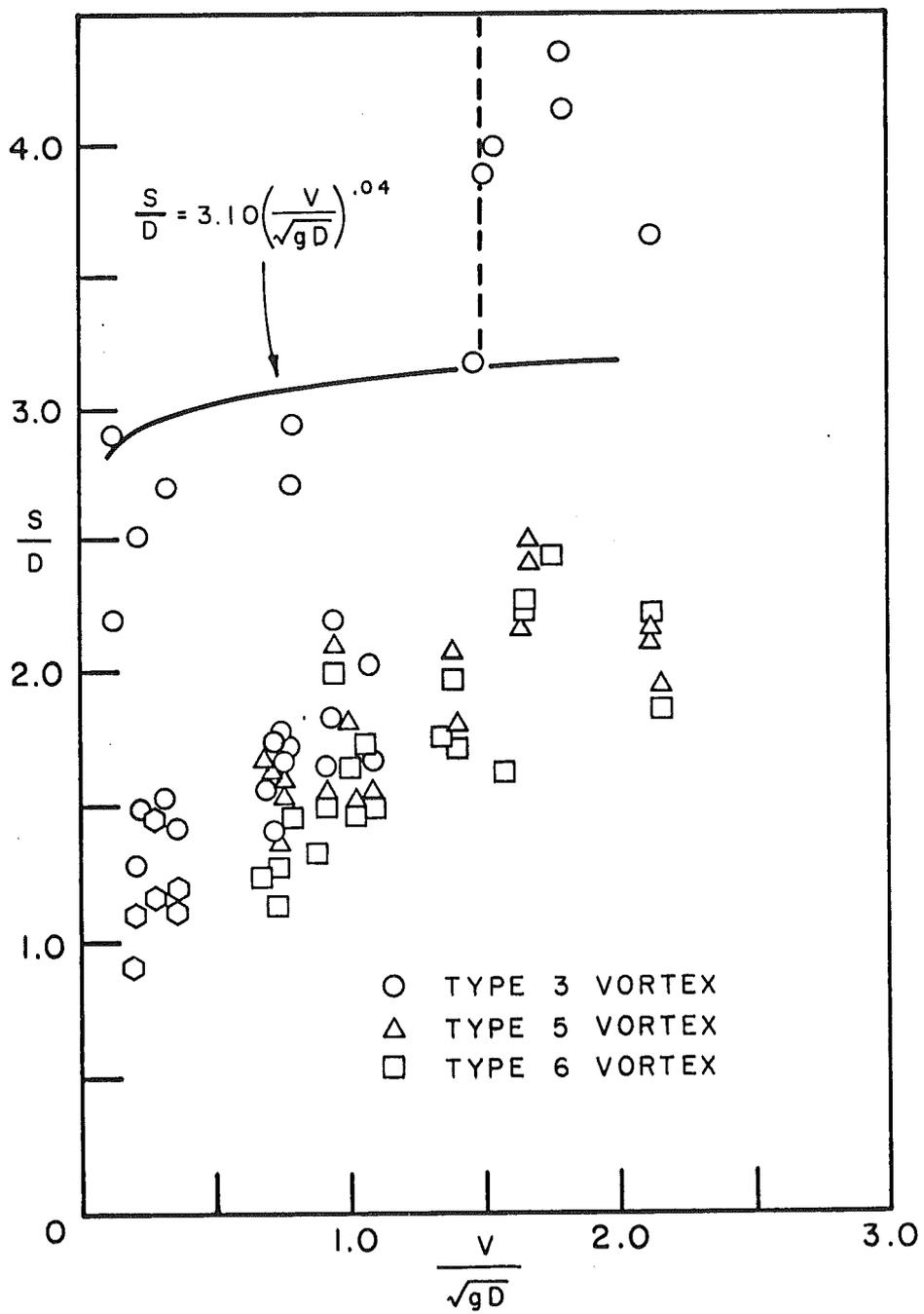
Fig. 35. Dimensionless submergence versus intake Froude number for  $15^\circ$  vane angle and  $L/W = 3.56$ . Hexagon symbol indicates viscous dimple.
