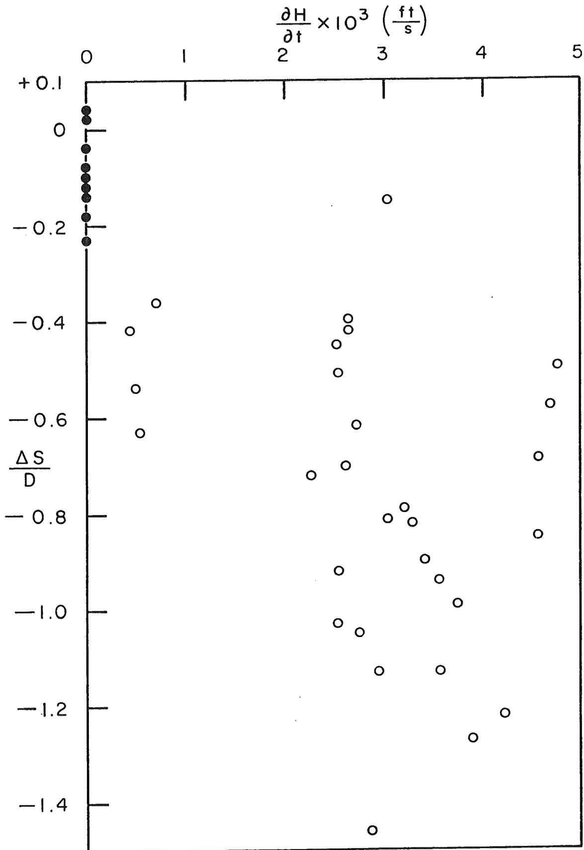
Fig. 37. Difference between actual measurements and envelope curve values of  $S/D$  versus rate of change of water surface elevation for Type 5 vortices. Open symbols - "on the run" measurements. Shaded symbol - steady water surface elevation.
