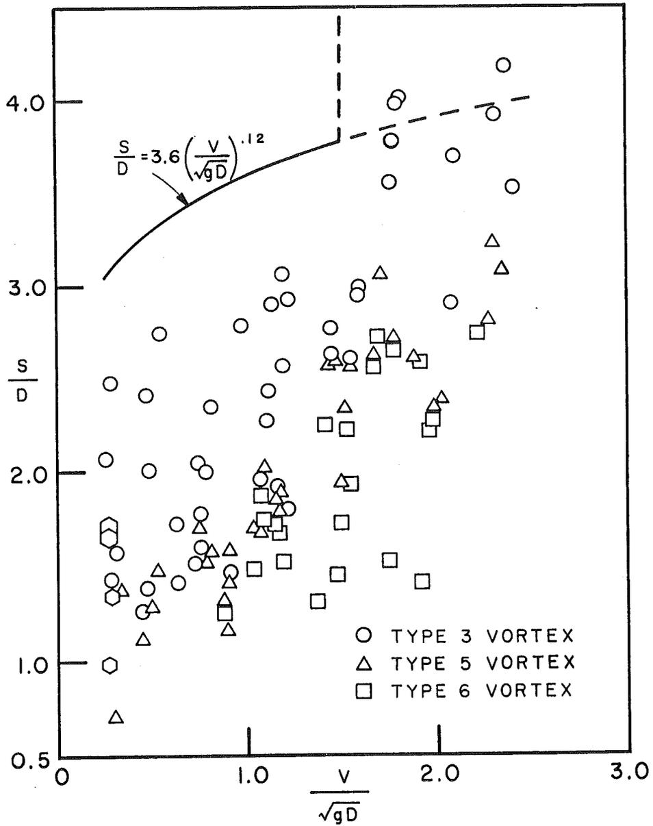
Fig. 26. Dimensionless submergence versus intake Froude number for  $0^\circ$  vane angle and  $L/W =$  channel length/width ratio = 1.13. Hexagon symbol indicates viscous dimple.
