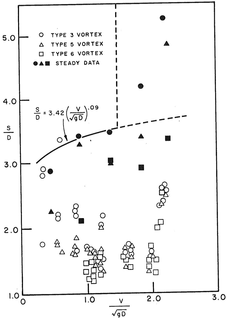
Fig. 30. Dimensionless submergence versus intake Froude number for  $0^\circ$  vane angle and  $L/W = 2.25$ .
