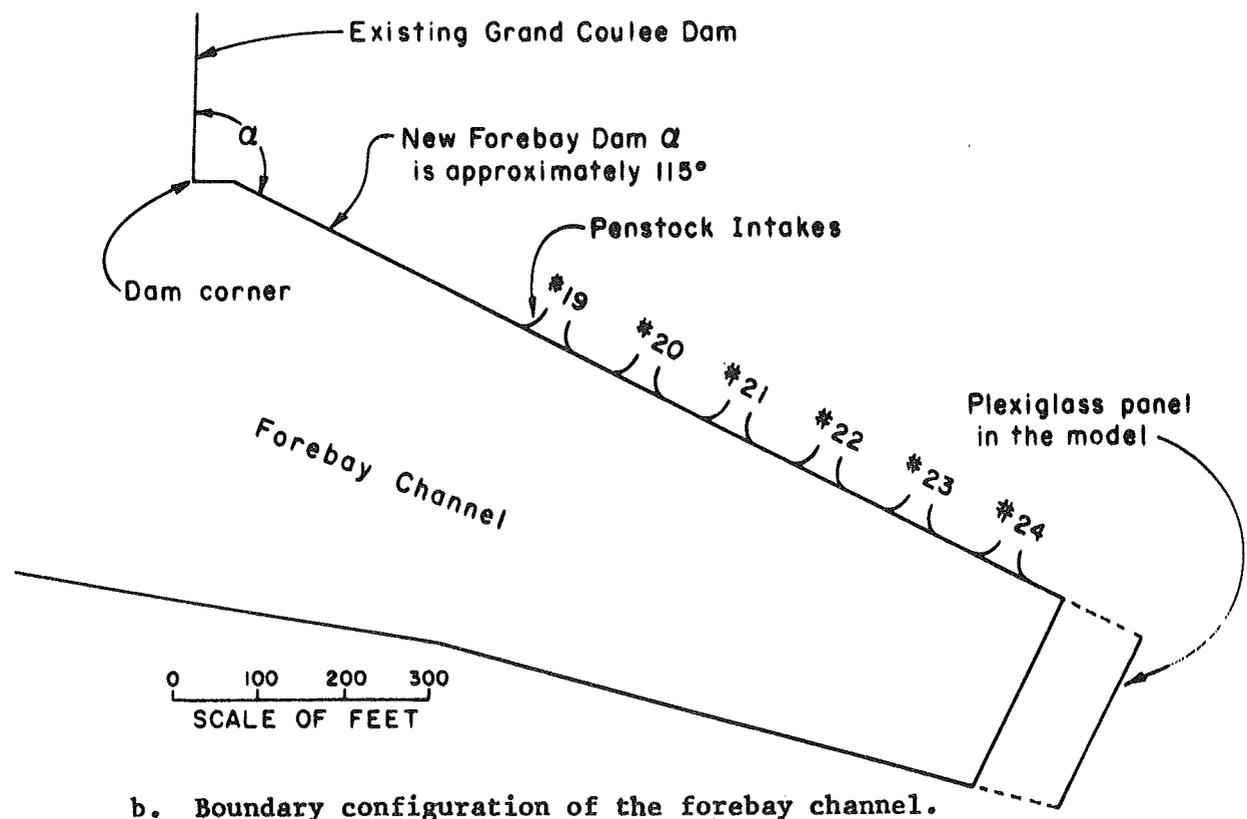
Fig. 12. Overall location sketch and location of intakes for Grand Coulee Third Power Plant, taken from Ziegler [20].
