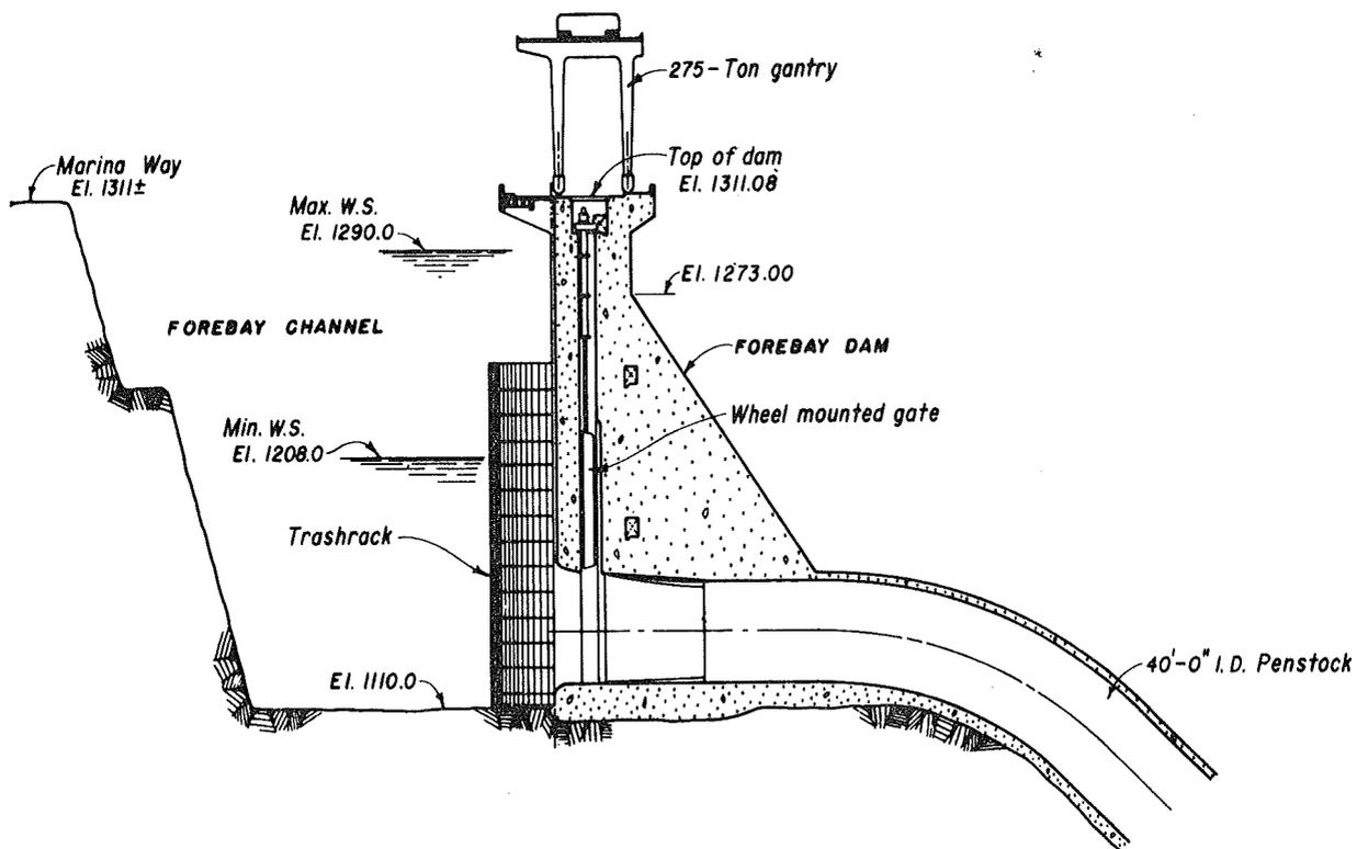
Fig. 13. Typical section view through forebay dam and penstock of Grand Coulee Third Power Plant, taken from Ziegler [20].
