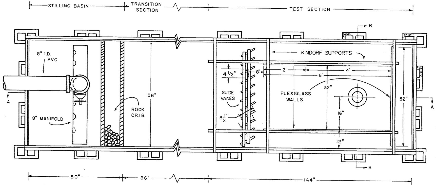
Fig. 20. Plan view of the experimental test facility.
