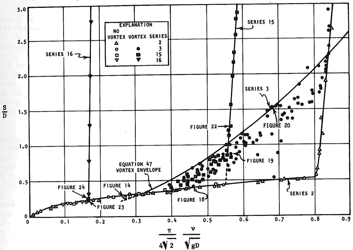
Fig. 4. Dimensionless submergence versus intake Froude number obtained from Humphrey et al. [17].
