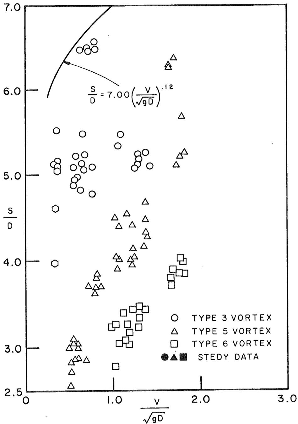
Fig. 29. Dimensionless submergence versus intake Froude number for  $30^\circ$  vane angle and  $L/W = 1.13$ . Hexagon symbol indicates viscous dimple.
