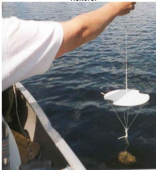
A new tool in 2004: a lightweight Secchi disk for use by Boundary Waters Canoe Area Wilderness visitors!
