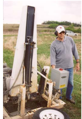
FIGURE 2. DNR hydrologists may use seismic equipment to assist with geologic mapping of potential aquifers. The seismic data complements existing well data.
