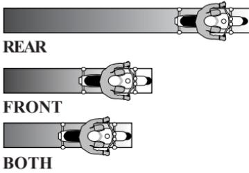
Always use both brakes at the same time to stop. The front brake can provide 70% or more of the potential stopping power.
