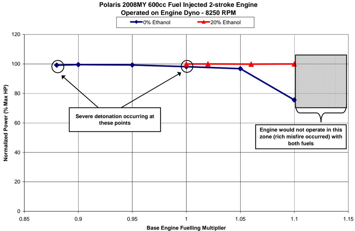
**Figure 8: 600cc 2-Stroke Fuel Sensitivity**
