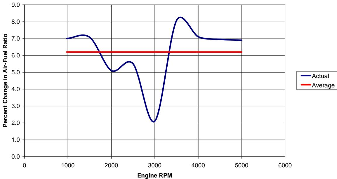
**Figure 5: Percentage Air-Fuel Ratio Change When Operating on E20 vs E0**
