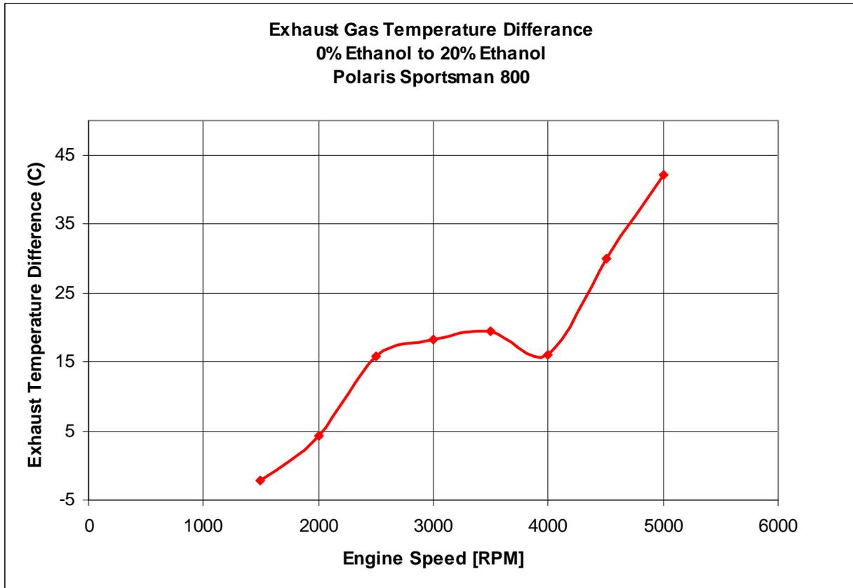
**Figure 3: Exhaust Gas Temperature Difference When Operating on E20 Compared to E0**
