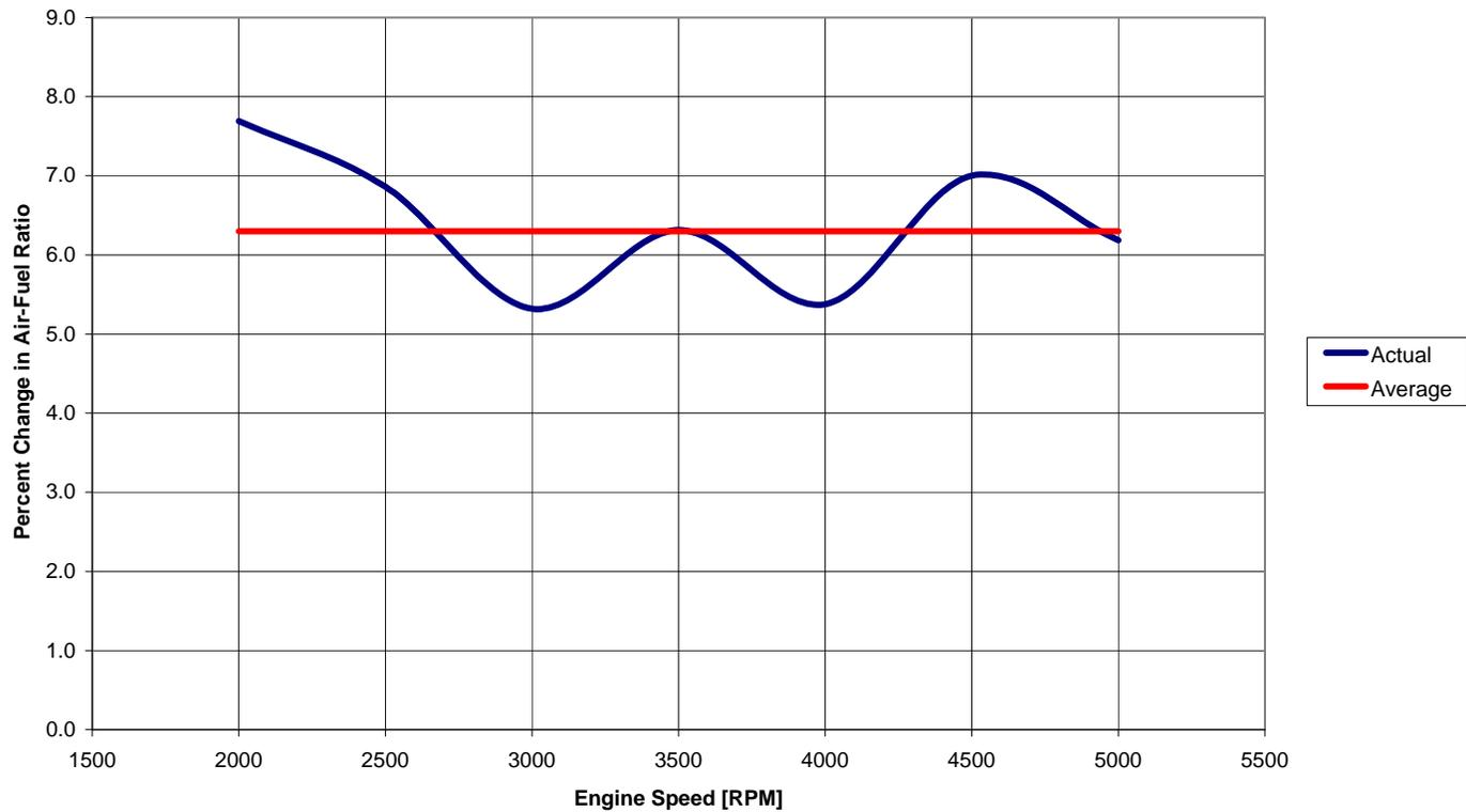
**Figure 2: Percentage Air-Fuel Ratio Change When Operating on E20 Compared to E0**
