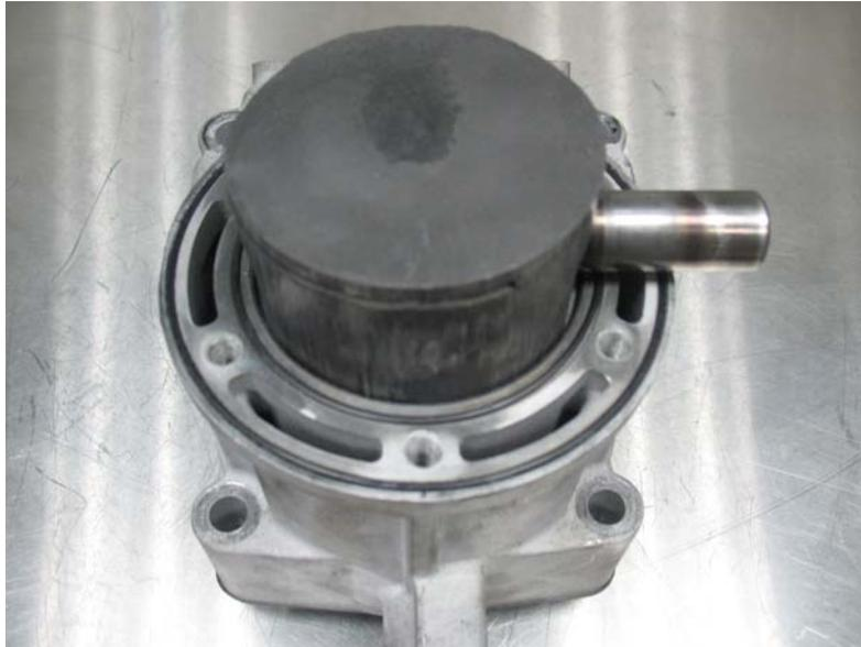
**Figure 9: 600cc 2-Stroke Piston Failure Due to Detonation**
