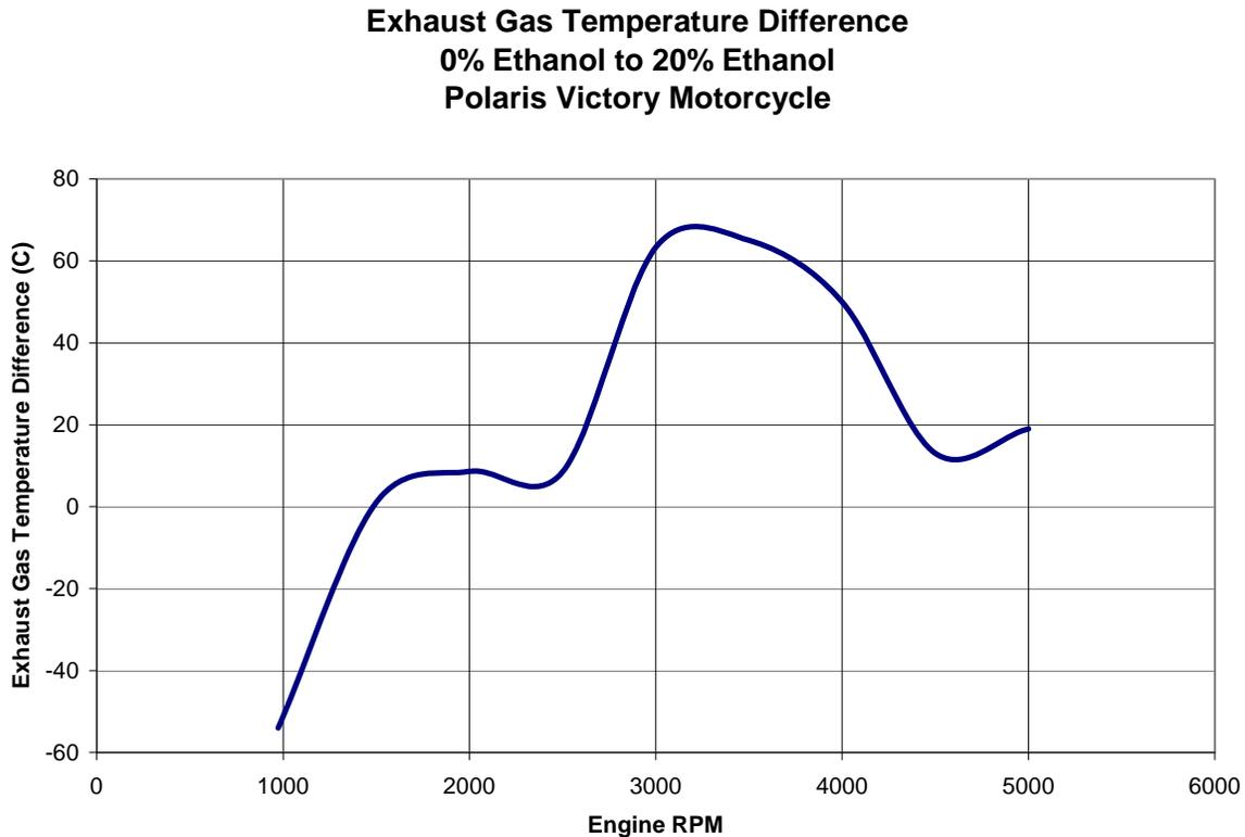
**Figure 6: Exhaust Gas Temperature Difference When Operating on E20 Compared to E0**
