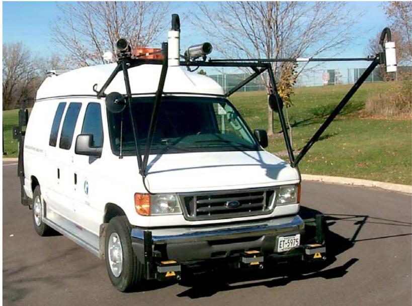
2005, a brand new van was put into service. This new van uses an improved rut measurement system. In 2006 and 2007, all eight districts were tested with this new van.
