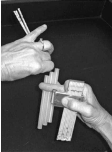
Figure 5.—Transferring 5 filled straws to each goblet, touching tips of straws only to avoid unnecessary warming. Pre-sealed ends of the straws must be inserted into the goblets, to avoid gumming up the goblets with loose sealant powder on the other end of the straws.
