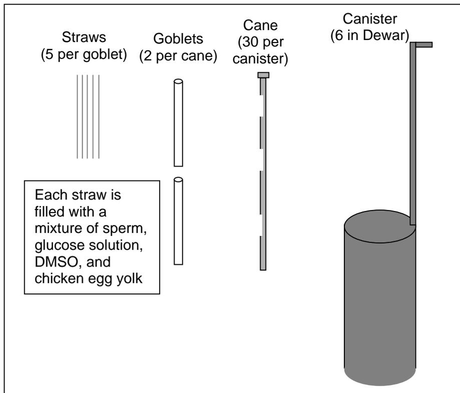
Figure 4.—Storage containers for cryopreserved sperm. Canisters are suspended in the liquid N<sub>2</sub> dewars. Ideally, straws are prepared in multiples of 10 from each sperm sample, filling 2 goblets on each cane, to use space efficiently. If a single goblet is stored in a cane, it should be positioned at the top of the cane to prevent straws from floating out of the goblet.
