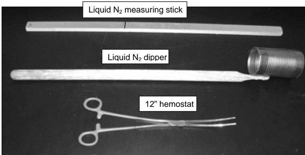
Figure 3.—Non-standard equipment used with liquid N<sub>2</sub>. The liquid N<sub>2</sub> measuring stick is made from a 2-foot stick, spray-painted, with “full” level marked. The liquid N<sub>2</sub> dipper is made from a soup can riveted to wooden net handle. The handle of the 12 inch hemostat has been dipped in Plastic Dip to facilitate handling with gloved fingers.
