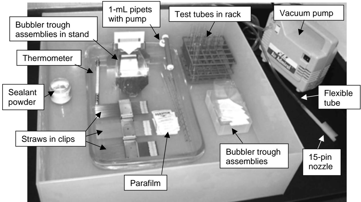
Figure 1.—Big Tray and working platform, with assembled materials.
