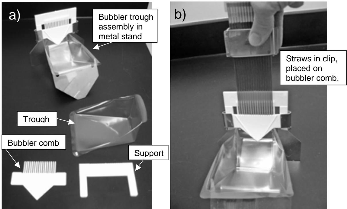
Figure 2.—a) Disposable “Bubblers trough assembly” (including trough, bubbler comb, and support) and metal stand. “Bubblers” refers to the 15-toothed plastic comb that is used to push some of the sperm sample out of each straw so that a bubble is formed, to allow expansion during freezing; b) Demonstration of 15 straws in a clip, fitted onto the straw comb.
