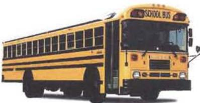
A "type D school bus" is constructed utilizing a stripped chassis. The entrance door is ahead of the front wheels.
