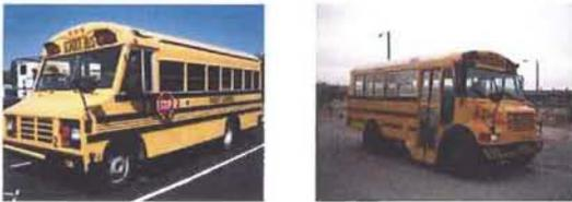
A "type B school bus" is constructed utilizing a stripped chassis. The entrance door is behind the front wheels. This definition includes two classifications: type B-I, with a GVWR less than or equal to 10,000 pounds; and type B-II, with a GVWR greater than 10,000 pounds.
