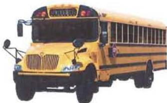
A "type C school bus" is constructed utilizing a chassis with a hood and front fender assembly. The entrance door is behind the front wheels.
