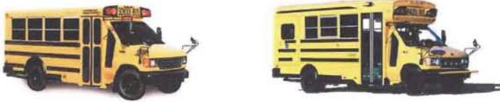
A "type A school bus" is a van conversion or bus constructed utilizing a cutaway front section vehicle with a left-side driver's door. The entrance door is behind the front wheels. This definition includes two classifications: type A-I, with a gross vehicle weight rating (GVWR) less than or equal to 10,000 pounds; and type A-II, with a GVWR greater than 10,000 pounds.
