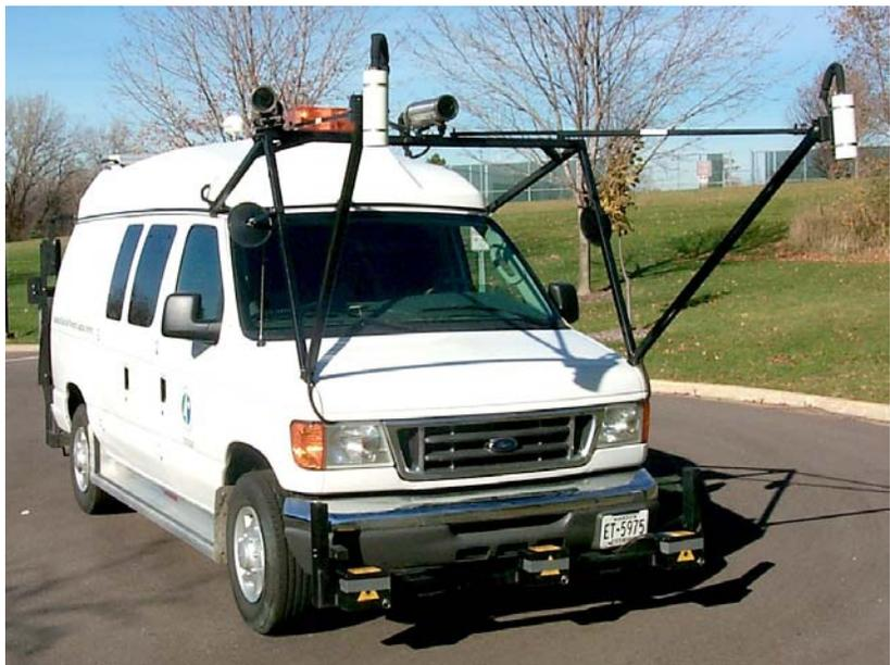
Pavement condition data is used to monitor the performance of the system, to help in the selection of projects, and identify pavements that need future maintenance and/or rehabilitation. The van drives over every mile of trunk highway annually, in both directions.
