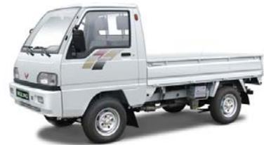
The trucks typically weigh between 1,400 and 1,800 pounds and have 12-inch wheels. Although they come in different forms, the standard is an open flat bed behind a small enclosed cab for the driver and one passenger. Most engines range from 550 cc to 660 cc and have 3 or 4 cylinders. Other features can include air conditioning and all-wheel drive. Uses of mini-trucks include
