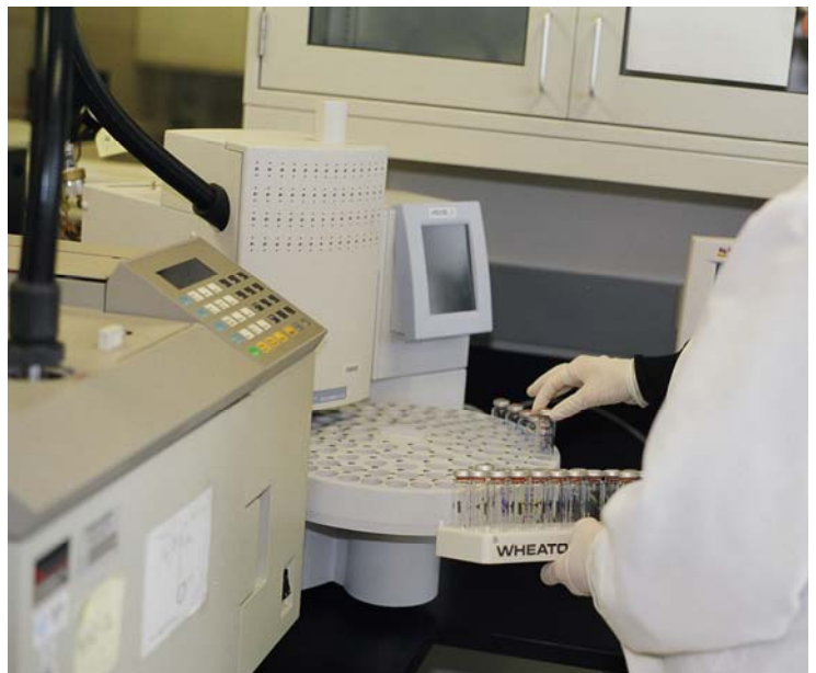
Loading Samples on a Headspace Gas Chromatograph
