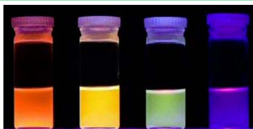
Professors Uwe Kortshagen (ME) and Steve Campbell (ECE) have developed silicon dots that luminesce. This could lead to efficient and environmentally benign lighting technologies.
