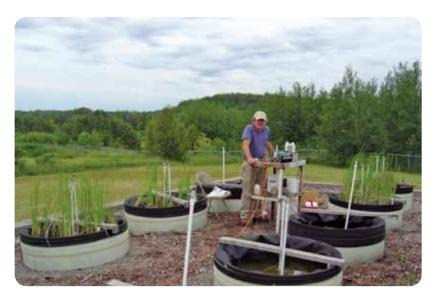
DNR staff study the use of alternative vegetation to protect drainage water from mining waste.
