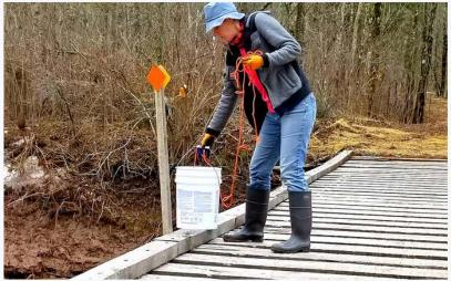
Torina Stark uses a bucket to get water to pour into a Secchi tube. Photo courtesy of Carlton SWCD
